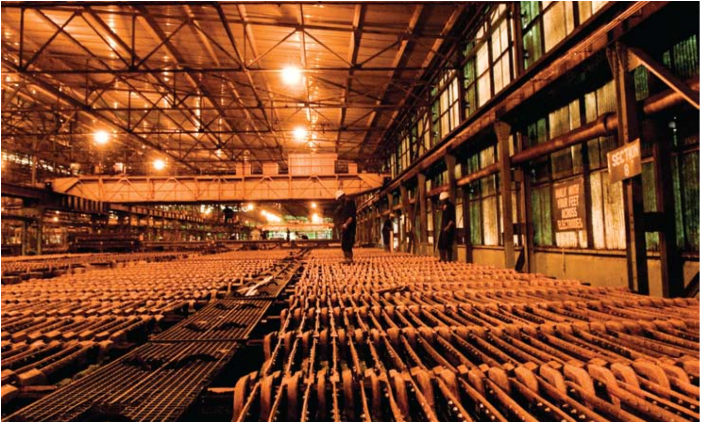
Copper electrowinning cells being processed into copper cathodes at the Tank House at Nchanga
