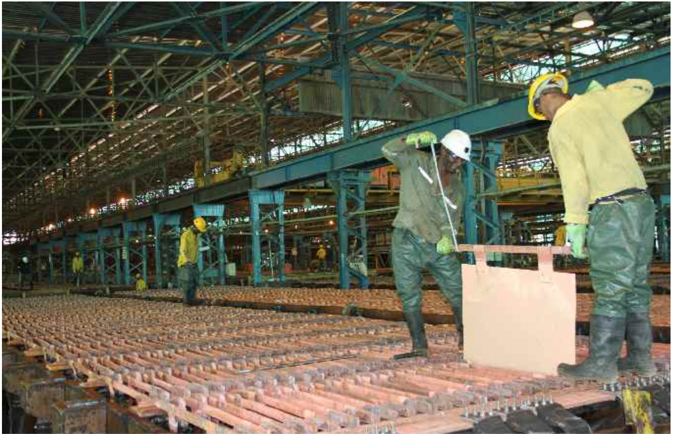
Employees on a routine inspection of the cells during electro refining process at Nkana Refinery
